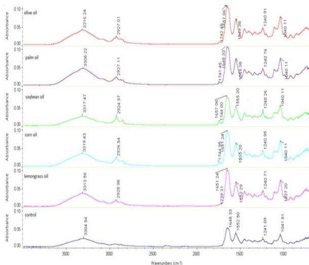
Figure 1. ATR-FTIR spectra of fish gelatin films incorporated with different vegetable oils.
